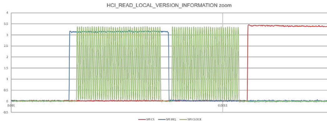
Figure 21. HCI_READ_LOCAL_VERSION_INFORMATION SPI waveform zoom
