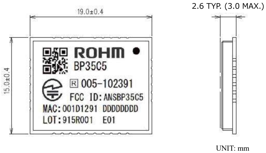
Fig. 3. Outline Dimensions Diagram
